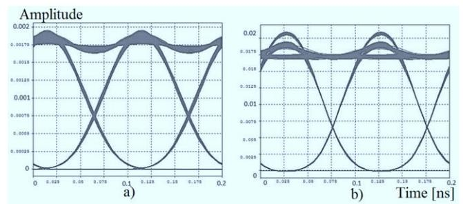
Fig. 8. The eye diagram for the simulation of SPM, CW laser power 0 dBm, CW power EDFA 0 dBm: a) *back\_to\_back* b) *received*
