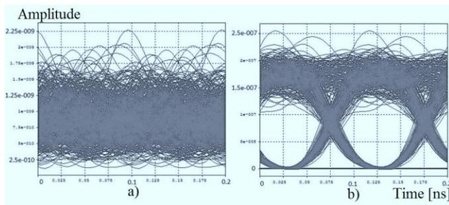
Fig. 9. The eye diagram for the simulation of SPM, CW laser power 80 dBm, CW power EDFA -80 dBm: a) *back\_to\_back* b) *received*
