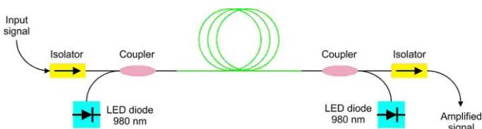
Fig. 5. The operating principle of a single EDFA
