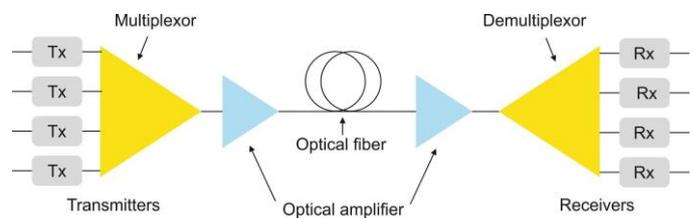
Fig. 1. The scheme of WDM technology
