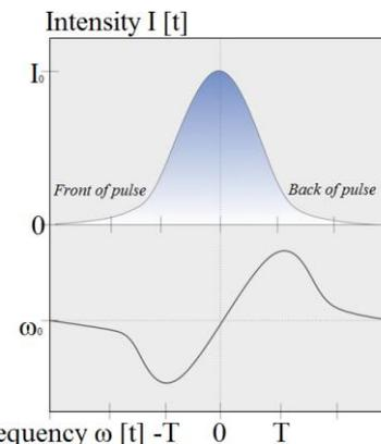
Fig. 4. Pulse frequency change due to SPM [8]
