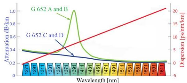
Fig. 3. CWDM channels defined by ITU – T G.694.2
