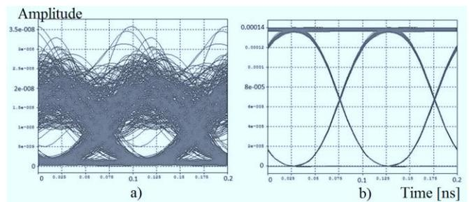
Fig. 7. The eye diagram for the simulation of SPM, CW laser power -80 dBm, CW power EDFA 80 dBm: a) *back\_to\_back* b) *received*
