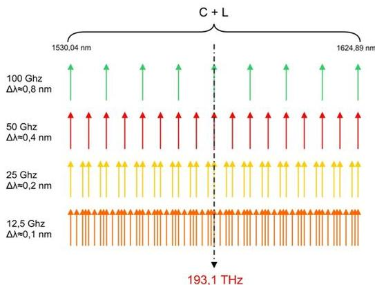
Fig. 2. The scheme of WDM technology
