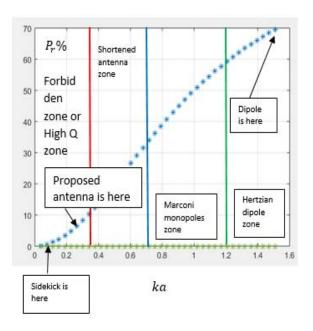
Fig. 6. Plotting the radiated power in percentages vs. ka using McLean formula (6)
