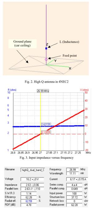
Fig. 4. The 4NEC2 program interface with the signal parameters at 26.99 MHz
