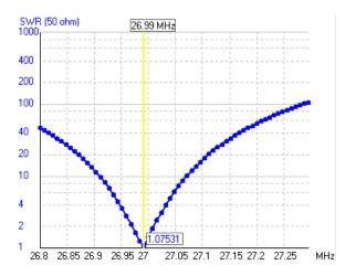
Fig. 6. The effect of the transformer over the VSWR (Voltage standing wave ratio)
