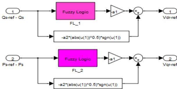
Fig.9 Structure of FSOSMC scheme.
