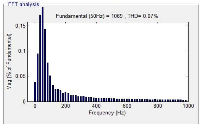
Fig. 22 Spectrum harmonic of stator current (FSOSMC-FSVPWM).
