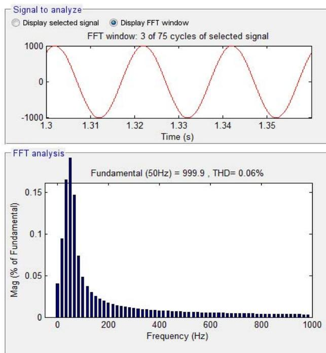
Fig. 14 Spectrum harmonic of stator current (FSOSMC-FSPWM).
