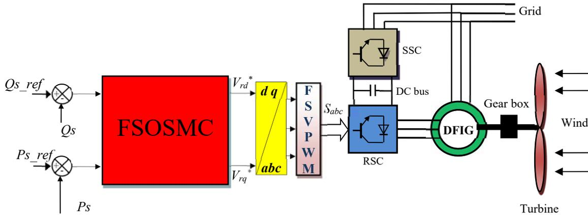
Fig. 8 FSOSMC block with FSVPM inverter.
