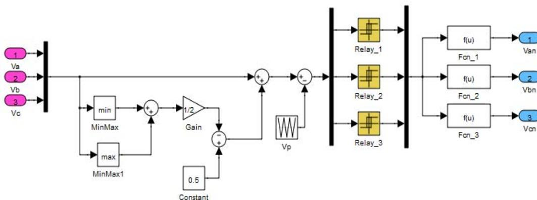
Fig. 1 Simulation block of proposed SVPWM technique.
