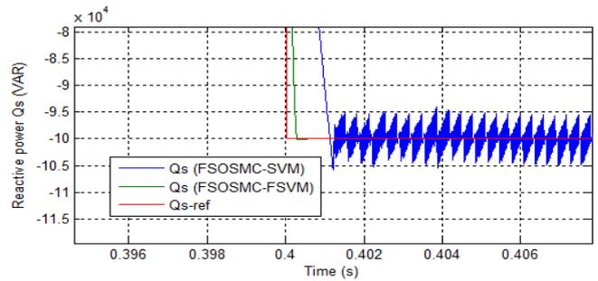
Fig. 16 Zoom in the reactive stator power (RTT).
