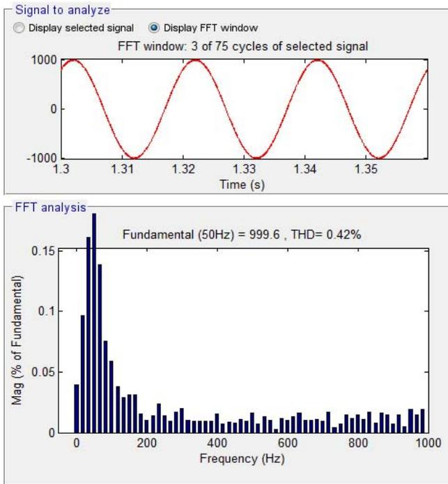
Fig. 13 Spectrum harmonic of stator current (FSOSMC-SVPWM).
