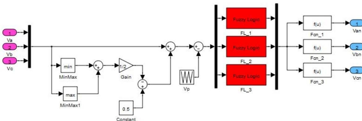
Fig. 2 SVPWM method with FL controllers.
